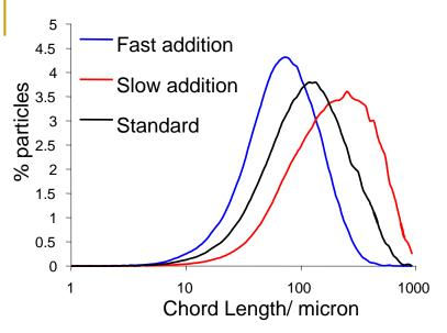
Process parameters investigated at laboratory scale mimic extremes of operating capabilities at commercial scale.
